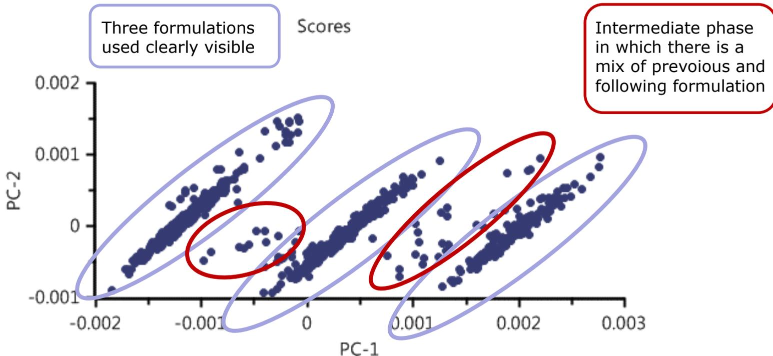
Spectra acquired during the batch production contains the information of the product flowing from the powder container to the die feeder of the tablet press.
