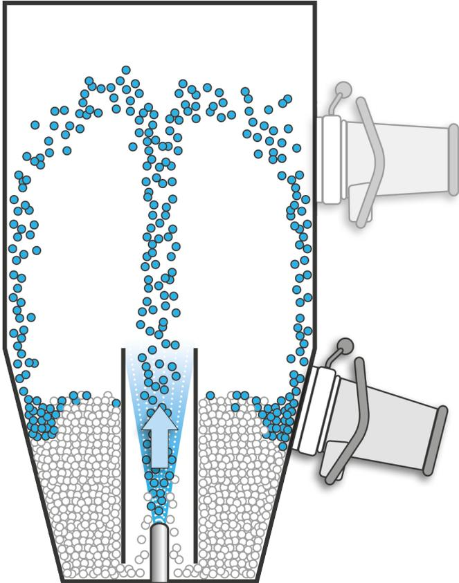
In-line and not-invasive monitoring of fluid bed pharmaceutical production processes.
